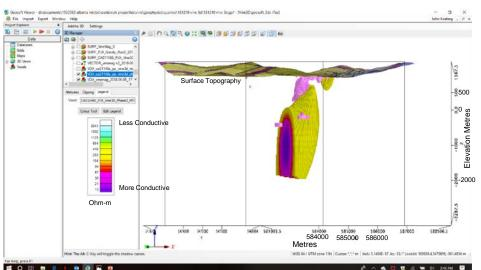
Cross Section through MT Targets and Magnetic Anomaly (3-Dimensional Image)
