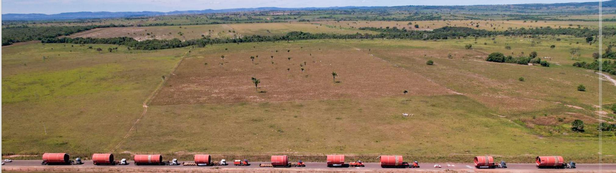
**“** The rotary kiln continues towards site. Here, convoys two and three (of four) make their way overland under a police escort. Each section weighs between 37 to 81 tonnes.
