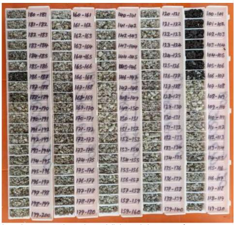
**Figure 3**: Visible spodumene zone observed in RC drill chips in hole GRC0670 from 107m to 187m with assays pending.
