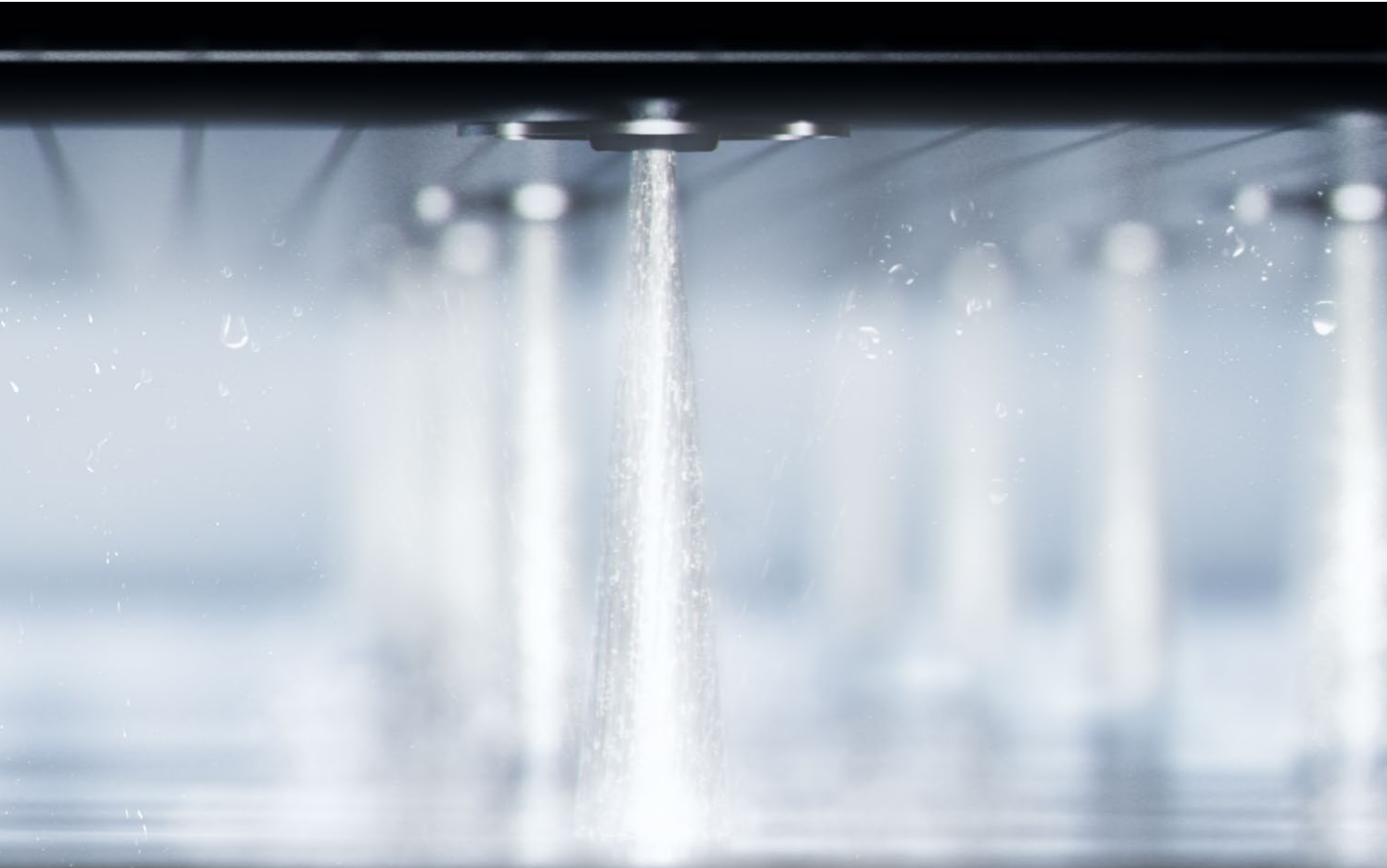
Image from Generation Phoenix demonstrating their hydro-entanglement process. Generation Phoenix has an on-site water treatment plant that enables them to recycle 95% of the water used to fuel the process.
