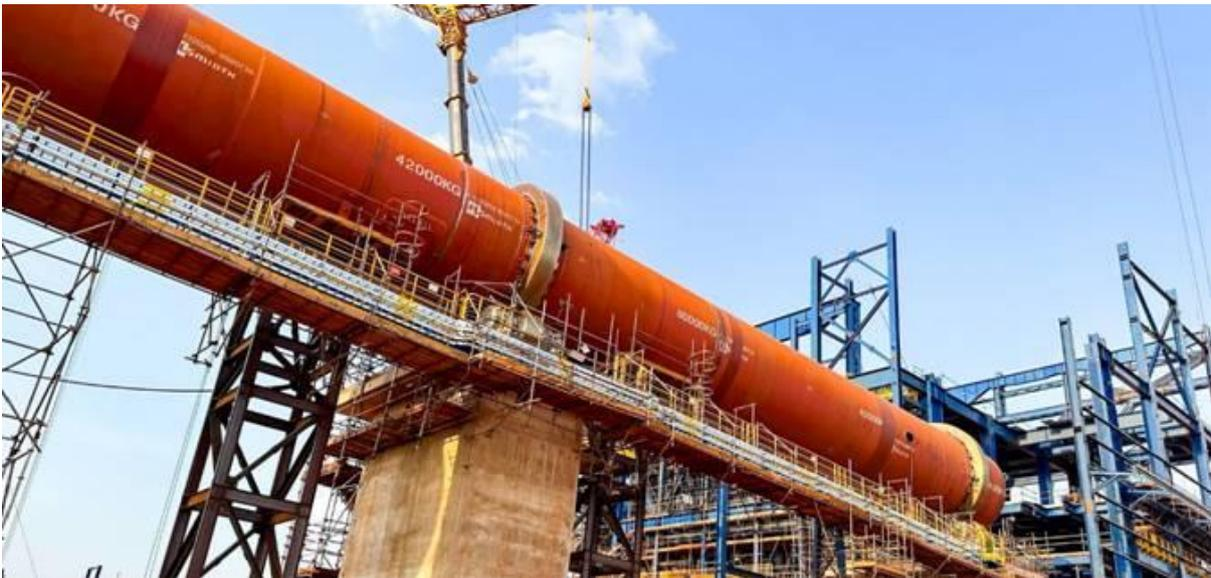
*The Rotary Kiln installed on the support piers with main roller bearing guide rings visible.*
