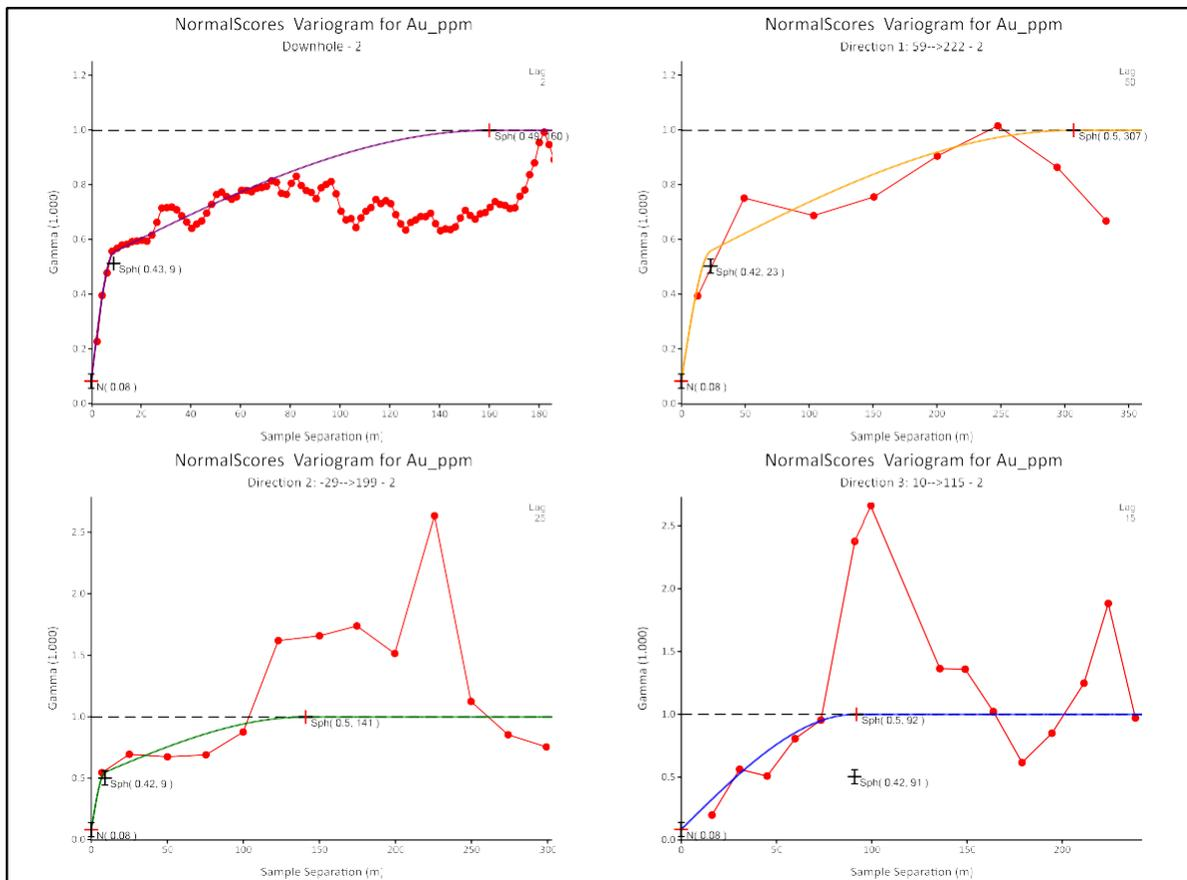
**Figure 14-12: Normalized variogram for Au in the domain 2**
