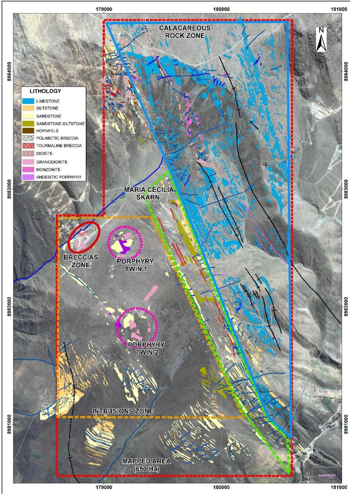
**Figure 7-10: Lithological map showing the breccia zone, the porphyry, the limestone zone, the skarn zone and the intrusive zone on the Maria Cecilia property.**
