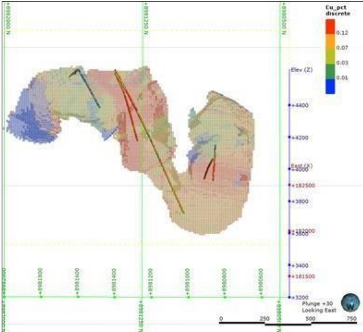
**Figure 14-14: Visual validation of Cu (%) block model in Emmanuel**
