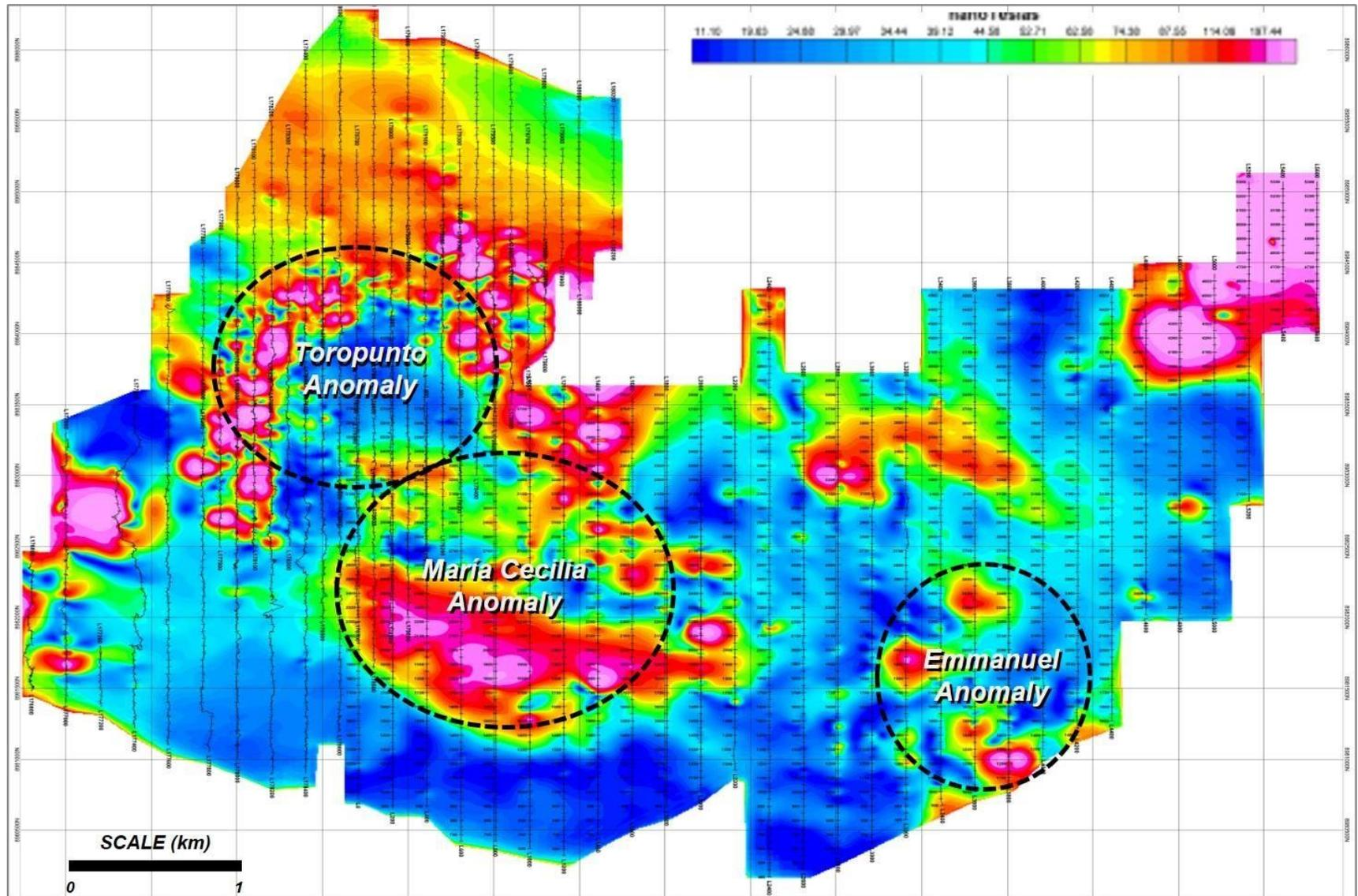
**Figure 1-1: Plan map of the combined magnetic surveys (total field), showing the approximate locations of the Toropunto, Maria Cecilia, and Emmanuel deposits with their respective magnetic anomalies.**
