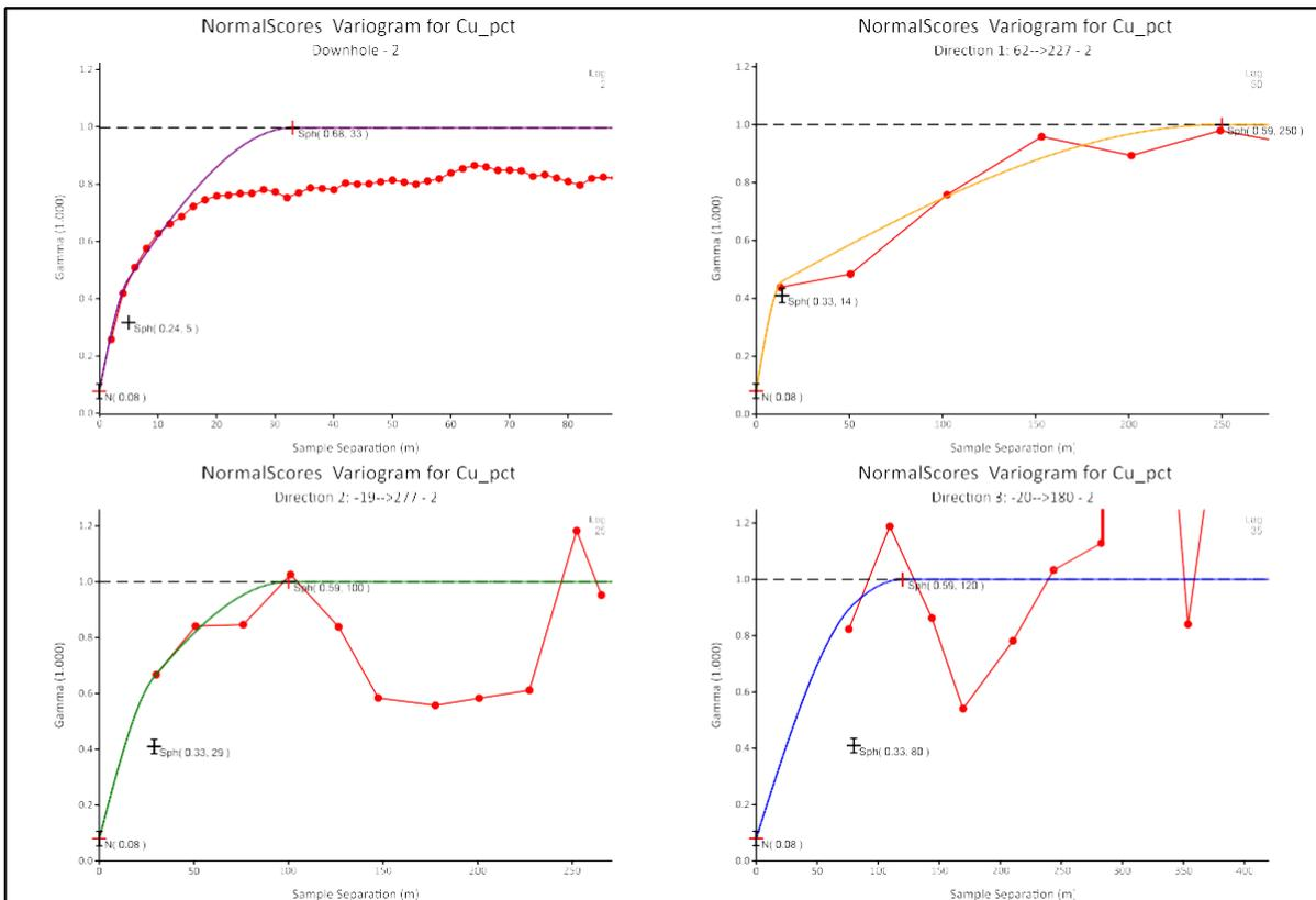
**Figure 14-8: Normalized variogram for Cu in the domain 2**
