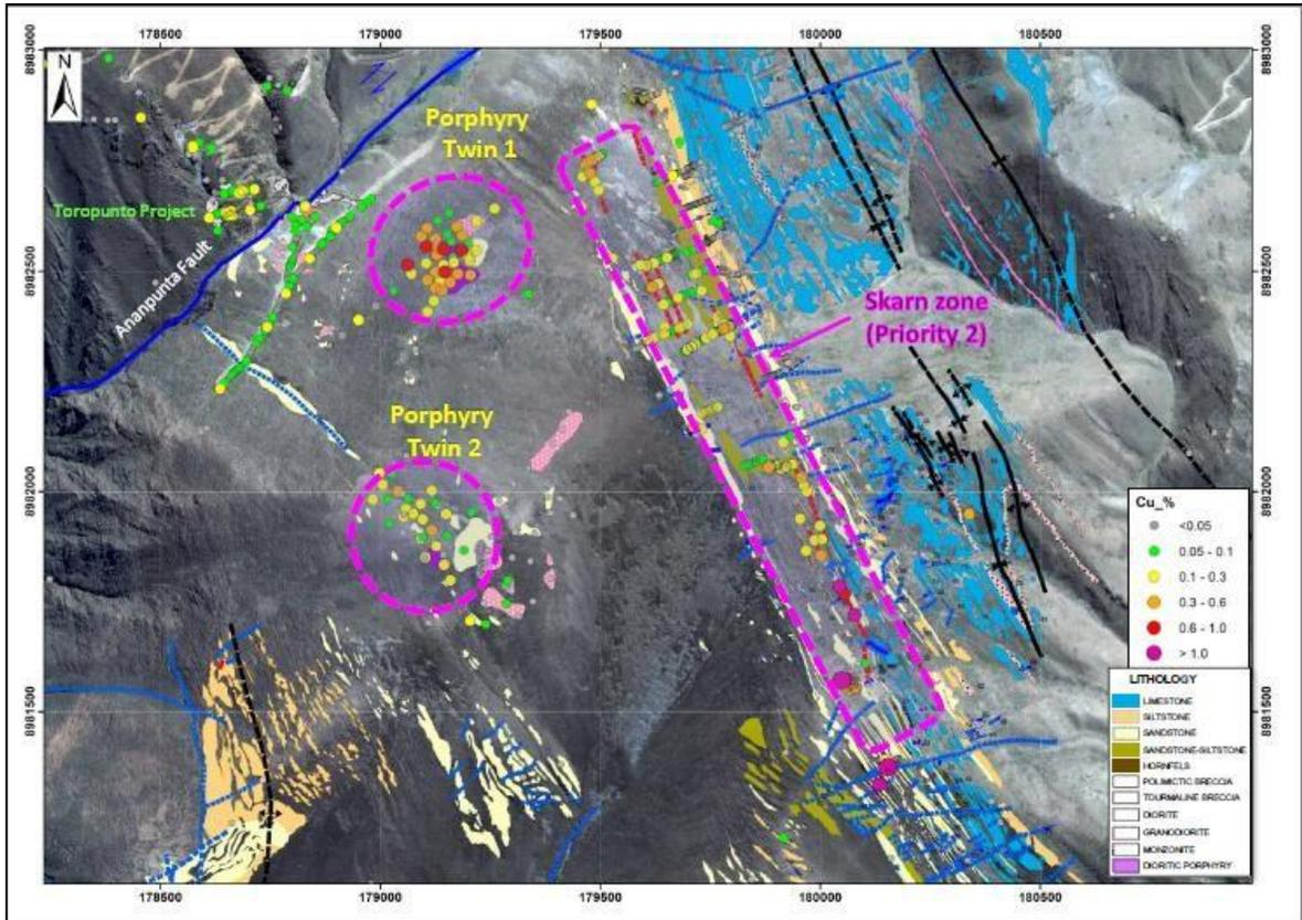
Figure 9-3: Plan view showing the lithological units of the Maria Cecilia project, surface geochemistry of Cu and the exploration targets (circles and discontinuous magenta boxes).
