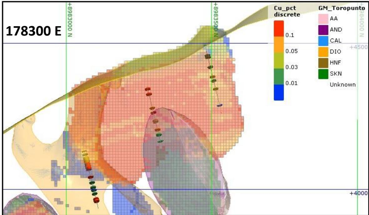
**Figure 14-10: Visual validation of Cu (%) from Toropunto block model**
