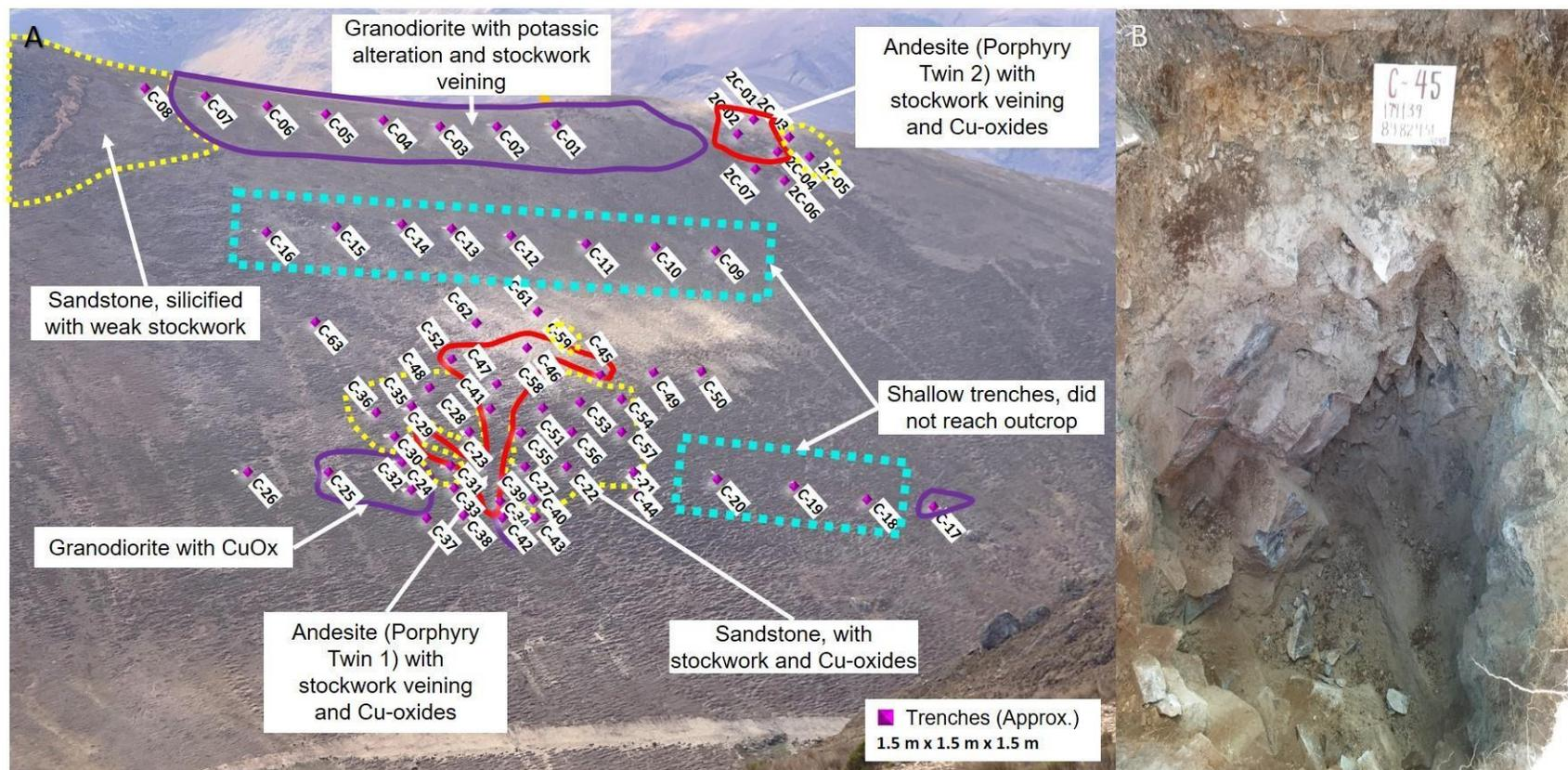
**Figure 9-4: Sampling (2019) at Maria Cecilia; (A) photograph looking to SE, showing approximate sample and/or trench locations (magenta boxes). Note approximate or inferred outline of silicified and/or weakly mineralized sandstone (yellow), granodiorite (purple-outline), and andesite porphyries (Twin 1 and Twin 2, red-outline), discontinuous blue-outline rectangles indicate samples/trenches that did not reach bedrock; (B) Example of excavated pit/trench (C-45).**
