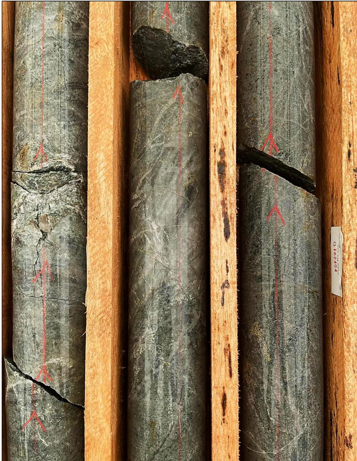
**Figure 5:** Selected drill core example of strong visible chalcopyrite copper sulphide mineralisation within a quartz-diorite intrusion in TAD-20-001. Drill core is HQ size or 63.5mm in diameter.
