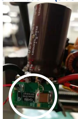
PFC with transition-mode controller L6562A (Side View)
