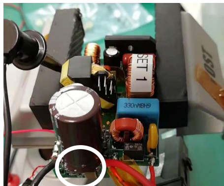
PFC with transition-mode controller L6562A (Top View)
