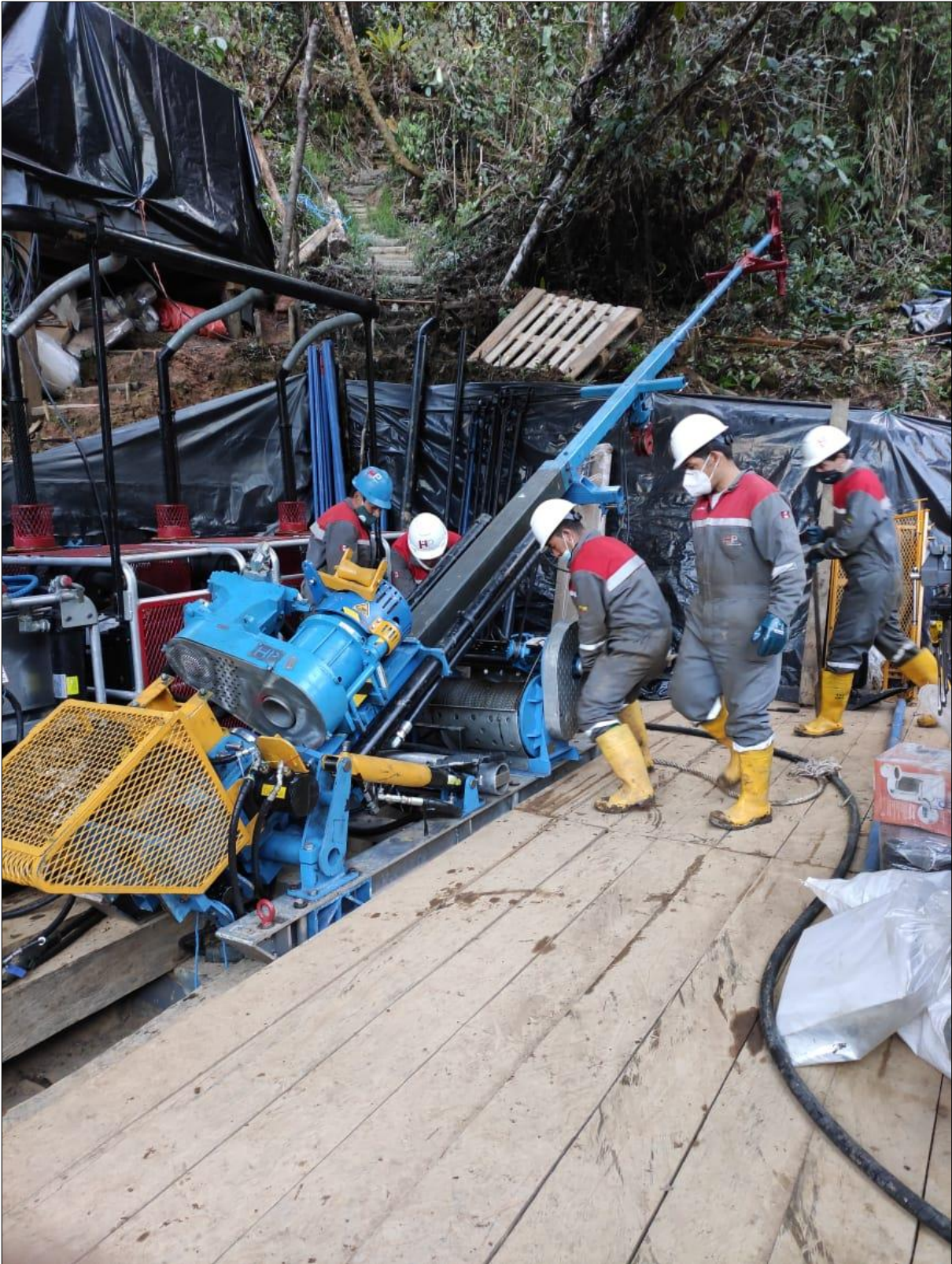
Figure 3: Hubbard Perforaciones drilling crew preparing commencement of Hole 1 (PDH-20-001) at Target 15, Porvenir, utilising a Hydracore™ 5000 hybrid man-portable machine modified to drill NQ sized diamond drill core up to 1800m depth.
