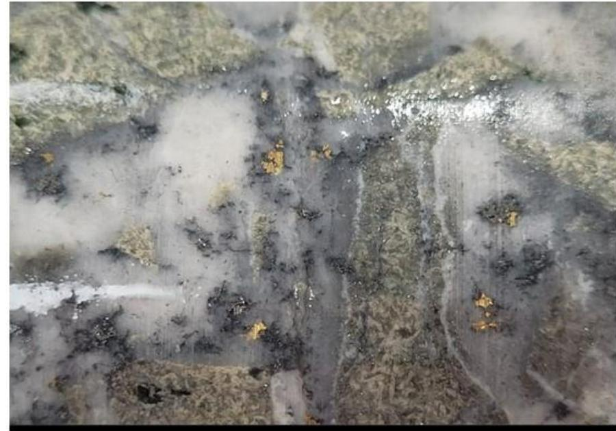
SDDSC077B from 739.9 m (0.8 m @ 1,741.5 g/t AuEq (1,736.4 g/t Au, 3.3% Sb) showing quartz-carbonate stockwork with visible gold, stibnite and sulphosalts in an altered dyke. Top to bottom 20 mm scale
