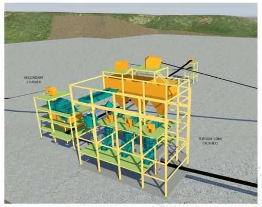
Figure 16: Secondary and tertiary crushing building
