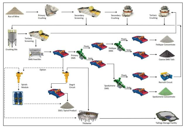
Figure 13: Overall simplified process flowsheet
