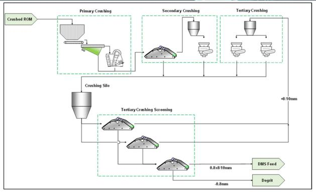
Figure 12: Crushing circuit flowsheet
