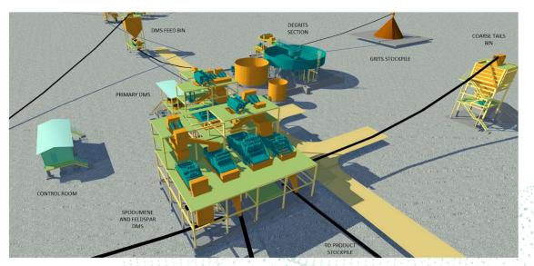
Figure 14: DMS plant layout showing key structures
