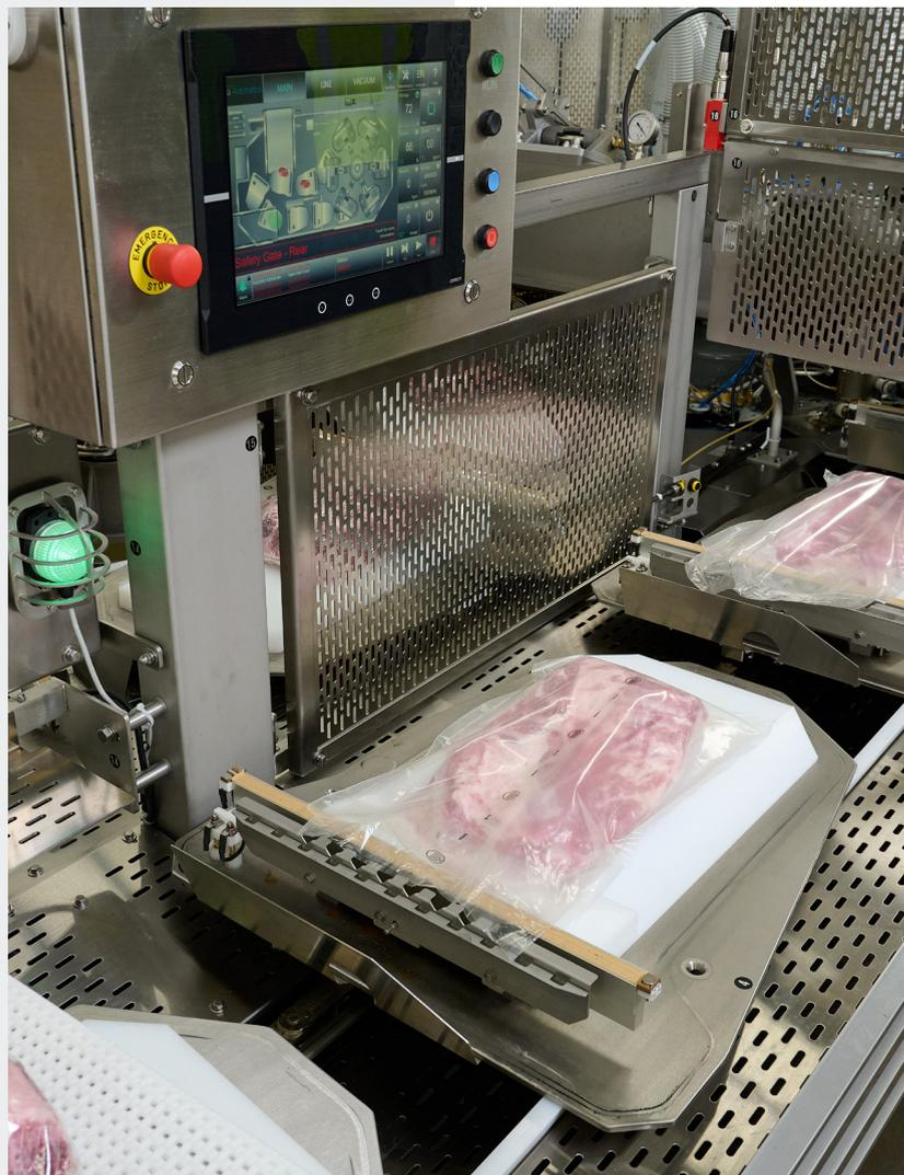
CRYOVAC® brand AutoVac 86 automated rotary vacuum chamber system
