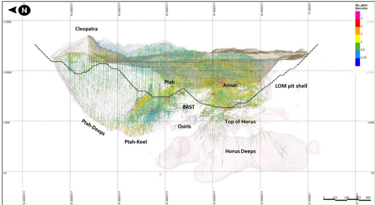
Figure 1: Long section looking east of the Sukari deposit, drill intercepts, the Sukari porphyry and extent of mineralisation with current and life of mine pit outlines.
