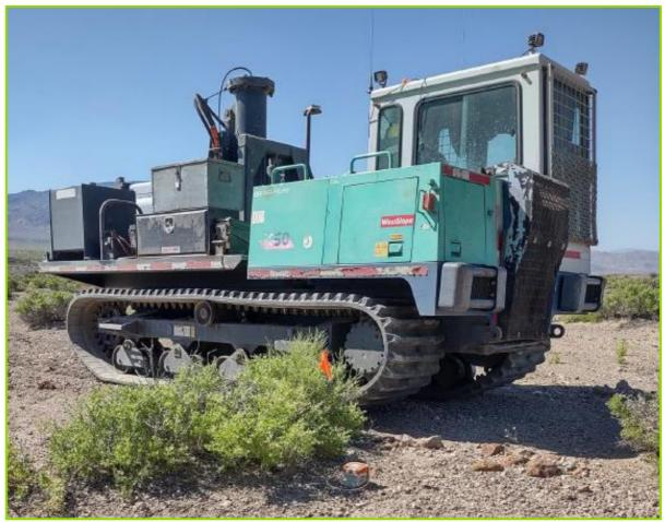
Figure 12: Accelerated weight drop seismic survey source.
