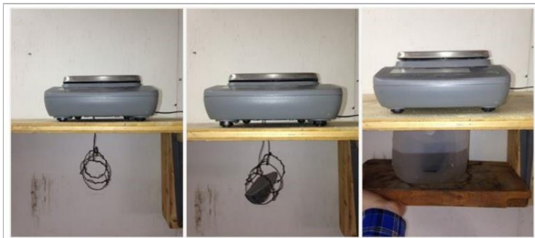
Figure 14-21: Specific Gravity Measurement Equipment Setup
