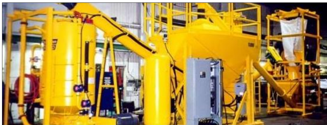
Figure 16-32: Illustration of a High-Shear Colloidal Cement Mixer
