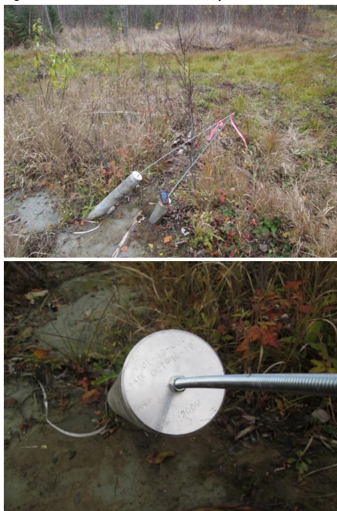
Figure 12-15: Miller Drillhole Collar & Cap for MI-19-35
