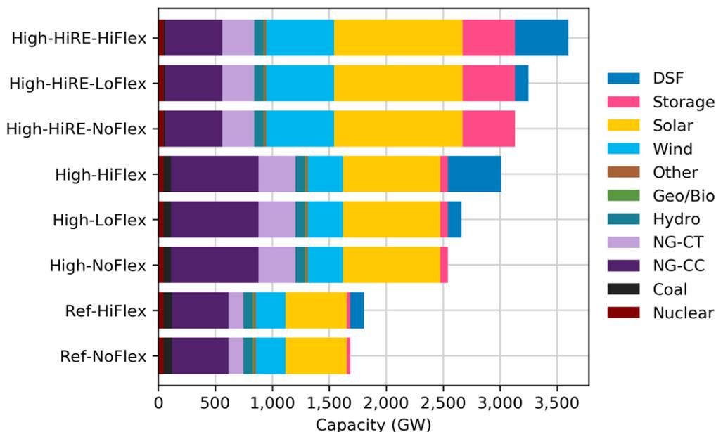
**Figure 6. Simulated 2050 installed generation capacity in the core scenarios<sup>26</sup>**
