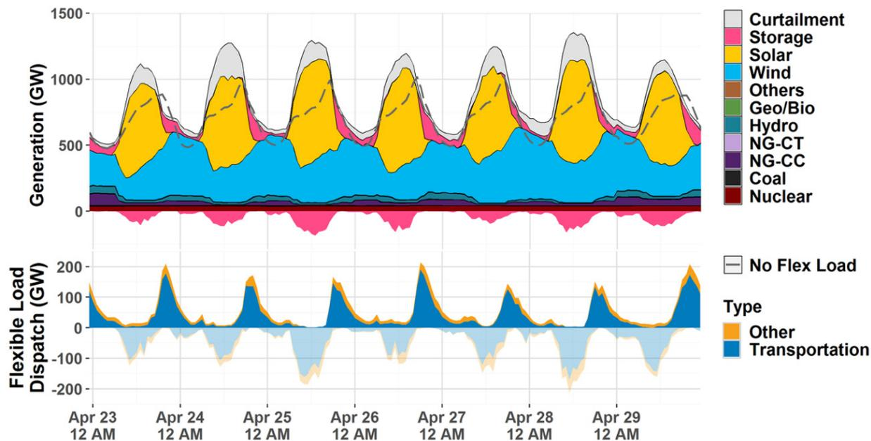
**Figure ES-1. Simulated 2050 generation (top) and flexible load (bottom) dispatch during a high-renewable period in spring under a high electrification scenario. Dash line indicates the original static load without demand-side flexibility. Pink portion below the X-axis indicates storage<sup>3</sup> charging.**
