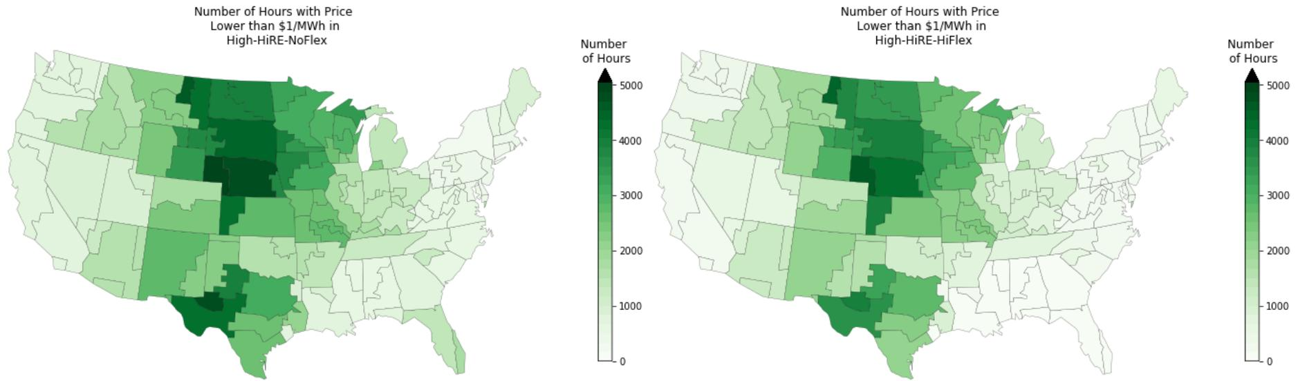
**Figure 31. Number of hours with price lower than \$1/MWh in High-HiRE-NoFlex (left) and High-HiRE-HiFlex (right) scenarios by balancing area**
