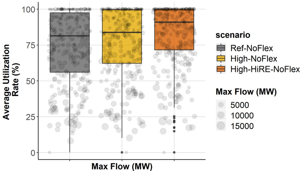
**Figure 12. Average interface transfer capability utilization rate distribution in the NoFlex scenarios**
