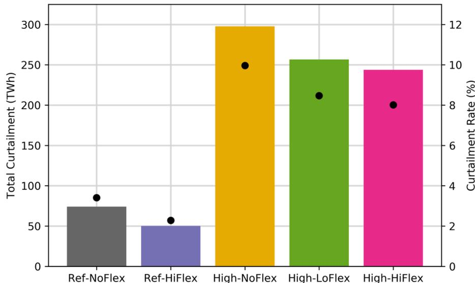
**Figure 24. Total curtailment (bars) and average curtailment rate (dots) in the Ref-NoFlex, Ref-HiFlex, High-NoFlex, High-LoFlex, and High-HiFlex scenarios**
