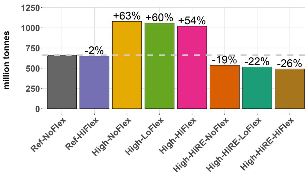
Figure 32. Annual power system CO<sub>2</sub> emissions (million tonnes) and difference from Ref-NoFlex emissions
