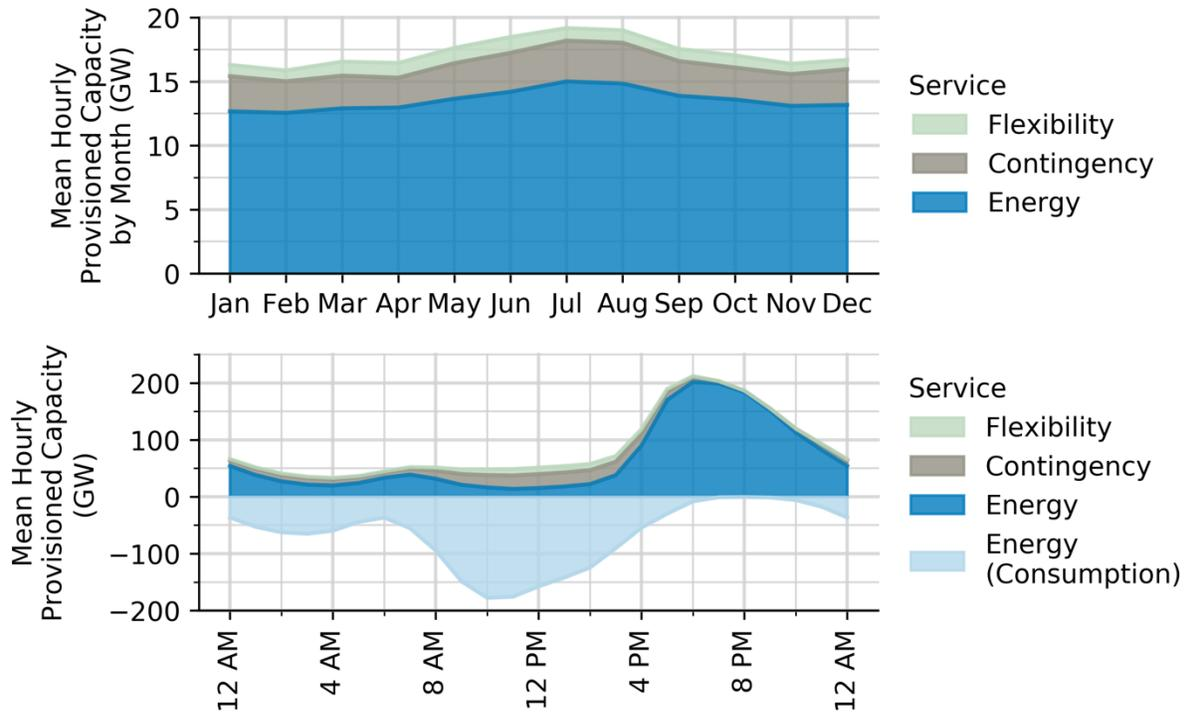
**Figure 19. Total DSF hourly mean provisioned capacity by service type by month (top) and by hour of the day (bottom) in the High-HiFlex scenario**
