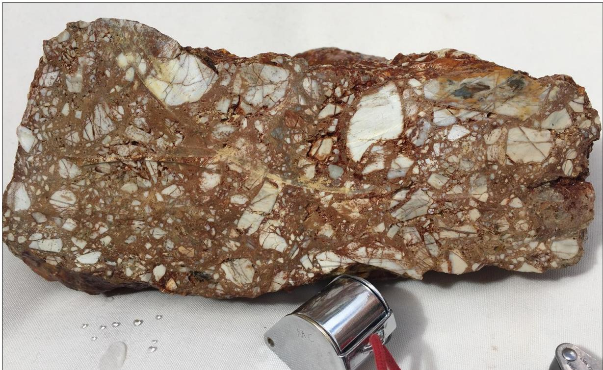
**Figure 10:** Example of gold bearing hydrothermal breccia containing clay altered lithocap fragments. This sample returned assay result of 1.0g/t Au.
