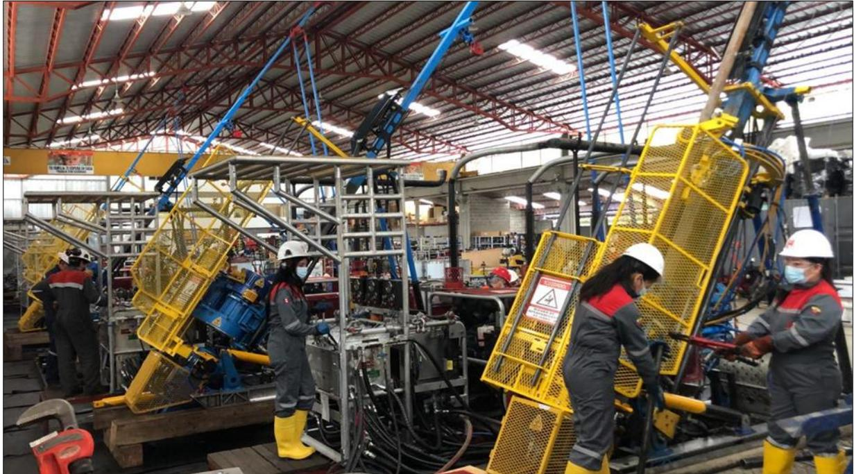
**Figure 3:** HP Drilling customised man-portable drill rigs being finalised at the HP Drilling workshop facility in Cuenca, Southern Ecuador. This work will continue as SolGold and HP Drilling work together to expand the fleet of diamond drill rigs for exploratory drilling at SolGold’s regional projects.
