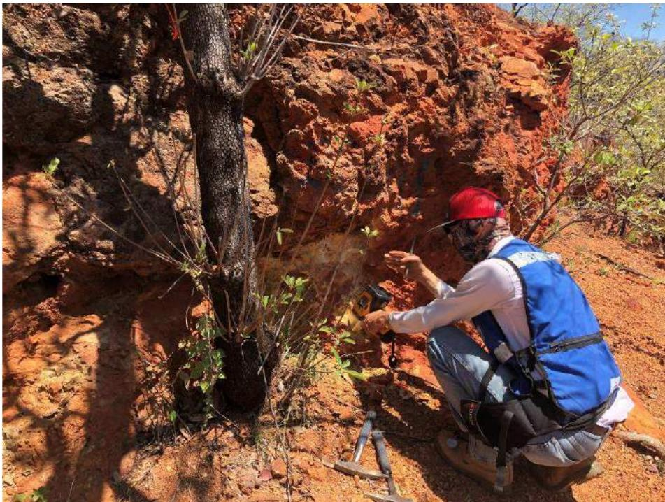
Taking XRF measurement at low angle breccia at Terrero near previous photo.
