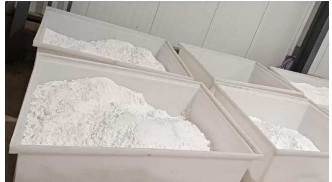
Figure 55: Li 2 CO 3 produced from batch operations during commissioning
