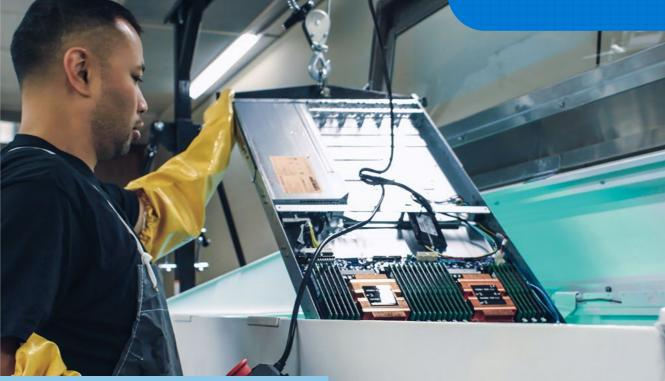
Advancing liquid immersion cooling technology helps to reduce water consumption in our operations.
